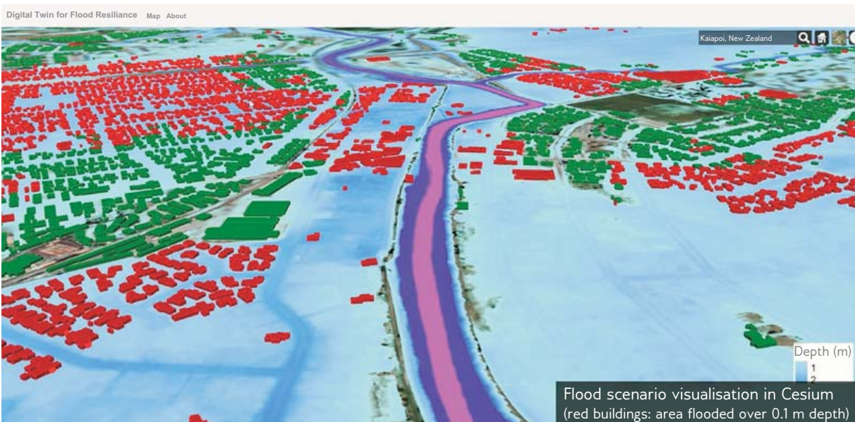
Figure 3: 3D visualisation from the prototype flood resilience digital twin, visualising flood levels in Kaiapoi, Canterbury. Buildings highlighted in red are flooded at a depth of 0.1 m or greater (Wilson, 2022).
