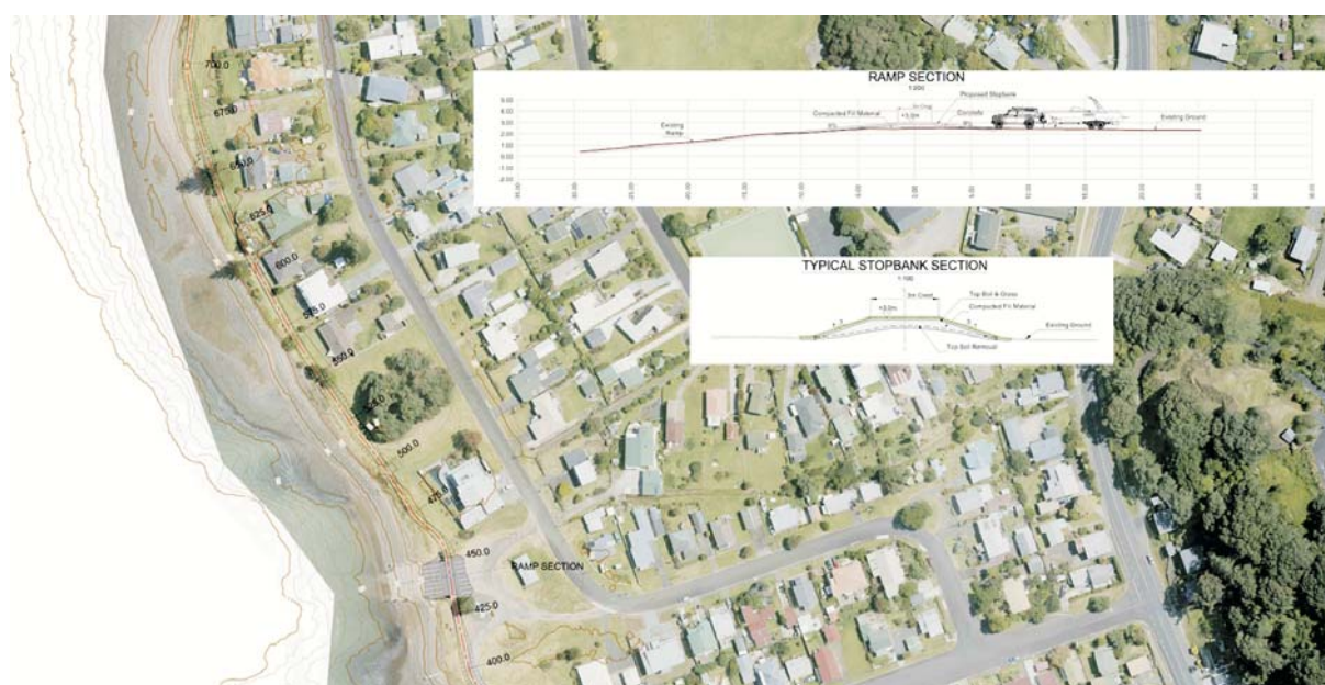
Figure 7: Concept design for the upgrade of the Te Puru coastal inundation defence (Source: IHBEYA).
