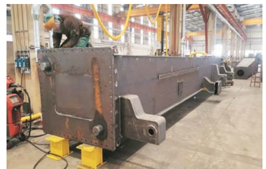
Travel lift under construction in Italy (Photo: Tauranga City Council).
