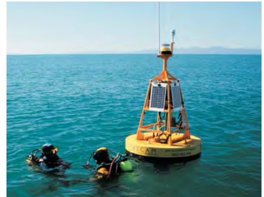
The TASCAM includes a buoy and instruments in the water column and on the seafloor below.
