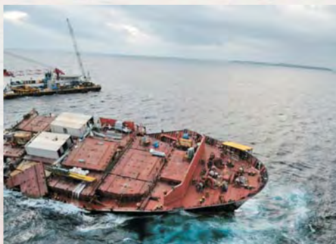
24 February, 2012: salvors have almost removed all of the containers from the top deck of the bow section of the Rena . Photo: LOC.
