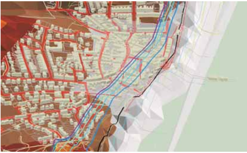
Figure 2: This image shows model predictions of cliff erosion at a town in Norfolk under a hypothetical scenario in which a cliff-toe seawall is removed. The bold lines indicate future predicted cliff positions at 10-year intervals between 2000 (black) and 2050 (purple). Roads are indicated by red lines, buildings by grey blocks, and a pier can be seen protruding into the sea on the right of the figure.
