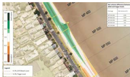
This image compares the current beach level with threshold levels documented in the beach scraping resource consent. Brown colouring highlights areas where sand levels are lower than consented threshold levels, and green areas show where beach scraping sand can be sourced (higher than threshold levels).
