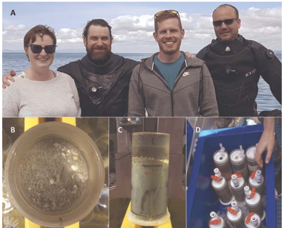
Figure 3: Photographs showing (A) members of the AUT/WRC project team and (B, C, D) acrylic tubes holding cores of FoT sediment. The team collects such cores at six sites featuring contrasting qualities of sediment.
