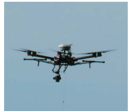
Trimble R8 GNSS receiver on the top of the DJI Matrice 600 drone (Photo: Maurice Perwick).
