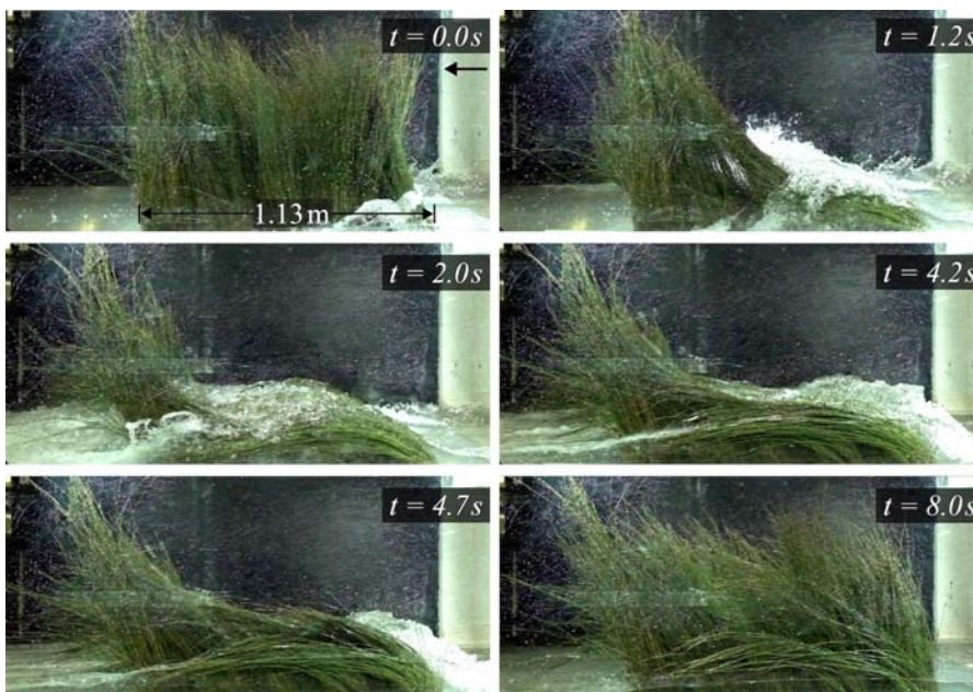
Figure 1: Five rows of oioi deflect in response to bore flow representative of wave overtopping. In the frame at t = 0.0 s, the arrow indicates the incident flow direction, and the dimension shows the array length. For this flow condition, the first few rows deflect until submerged, while the downstream rows remain emergent. The oioi then returns to approximately its original position.
