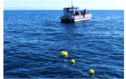
Figure 1: Wave buoys deployed off Bethells Beach (west coast), and in the Hauraki Gulf.
