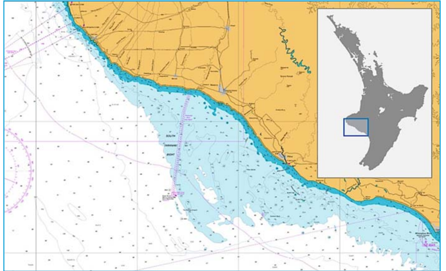
Figure 1: South Taranaki Bight, from LINZ Chart 45. Dark blue area shows 0-10 m water depth, light blue area shows 11-30 m water depth, white area shows > 30 m water depth, CMA boundary (12 nm) shown with thin pink line.
