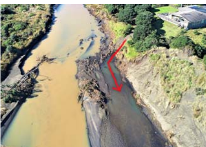
Figure 4: Post flood event, vehicle accessway washed away (access route identified in red).
