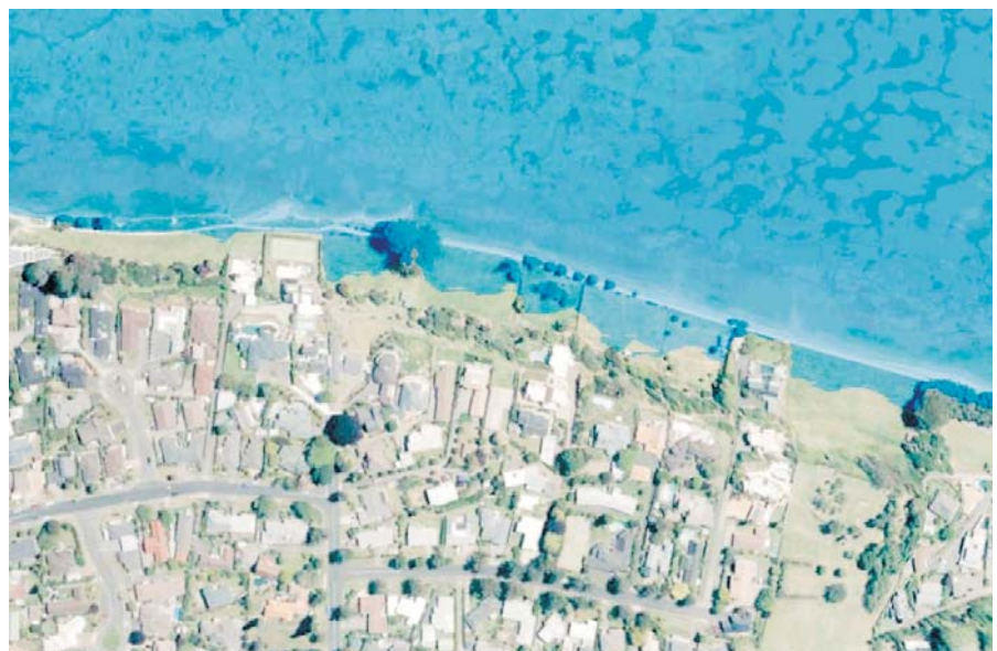
Figure 6: Example of bathtub inundation using extreme water level predictions (2.1 m MVD) and 2015 LiDAR.
