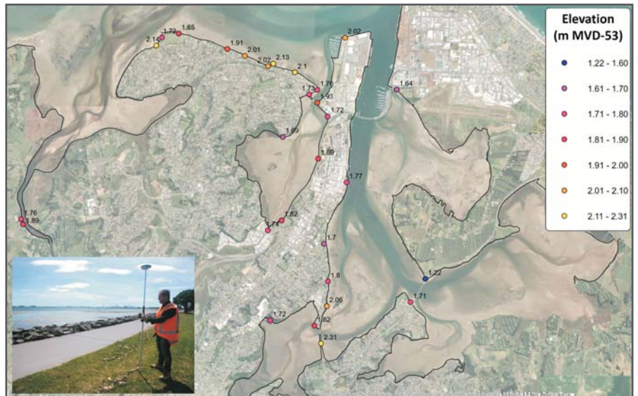
Figure 3: Location and elevation of debris lines recorded after the 5 January 2018 event.
