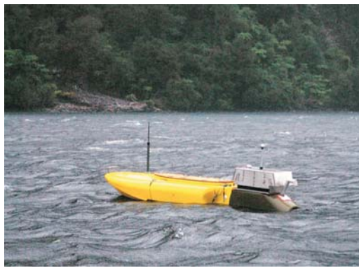
Oregon State University autonomous surface vessel ROSS houses a 10-metre-long instrument chain that profiles as it goes, as well as an acoustic current profiler. Photo: Craig Stevens, NIWA.
