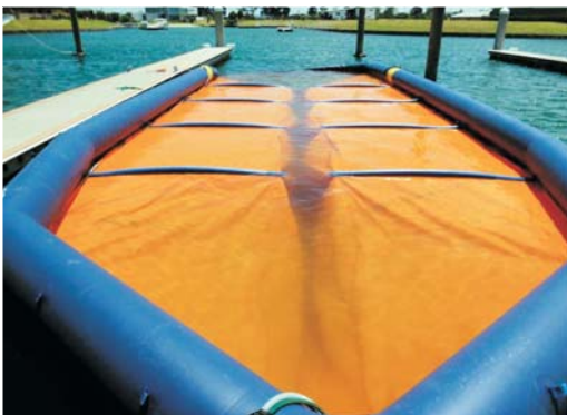
The VQF can quarantine a vessel up to 16 m in length. Photo: NRC.
