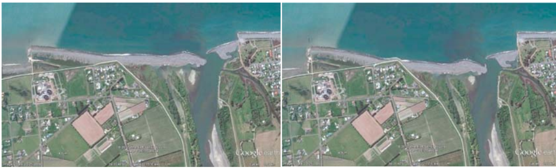
Figure 1 (left): Predicted coastline after 50 years with no Haumoana groyne scheme; Figure 2 (right): Predicted coastline after 50 years with the Haumoana groyne scheme (no mitigation or prefill). Figures: HBRC.
