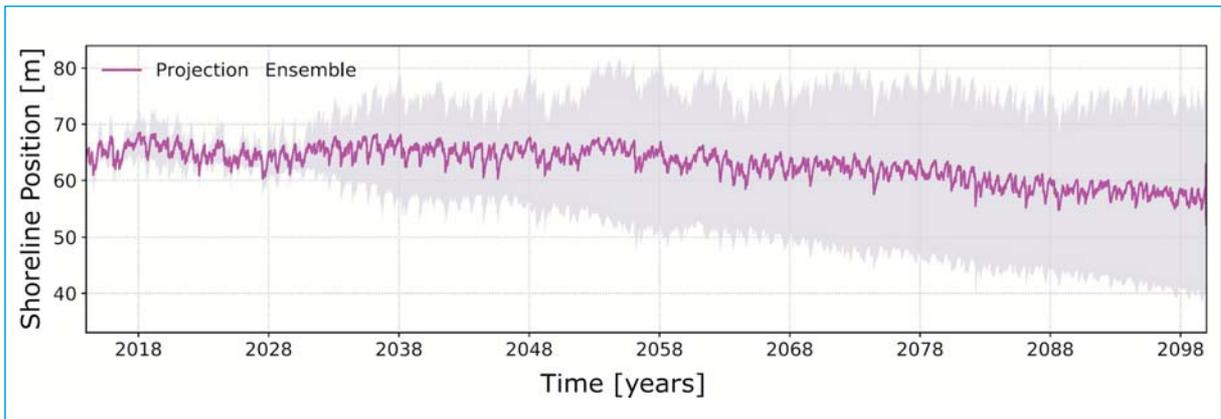
Figure 2: Prediction of shoreline position at Tairua beach under sea level rise. Lower values of shoreline position indicate erosion (initial shoreline position is at about 65 m). The thick line shows the ensemble of different shoreline evolution models while the shaded area shows the standard deviation around the ensemble.
