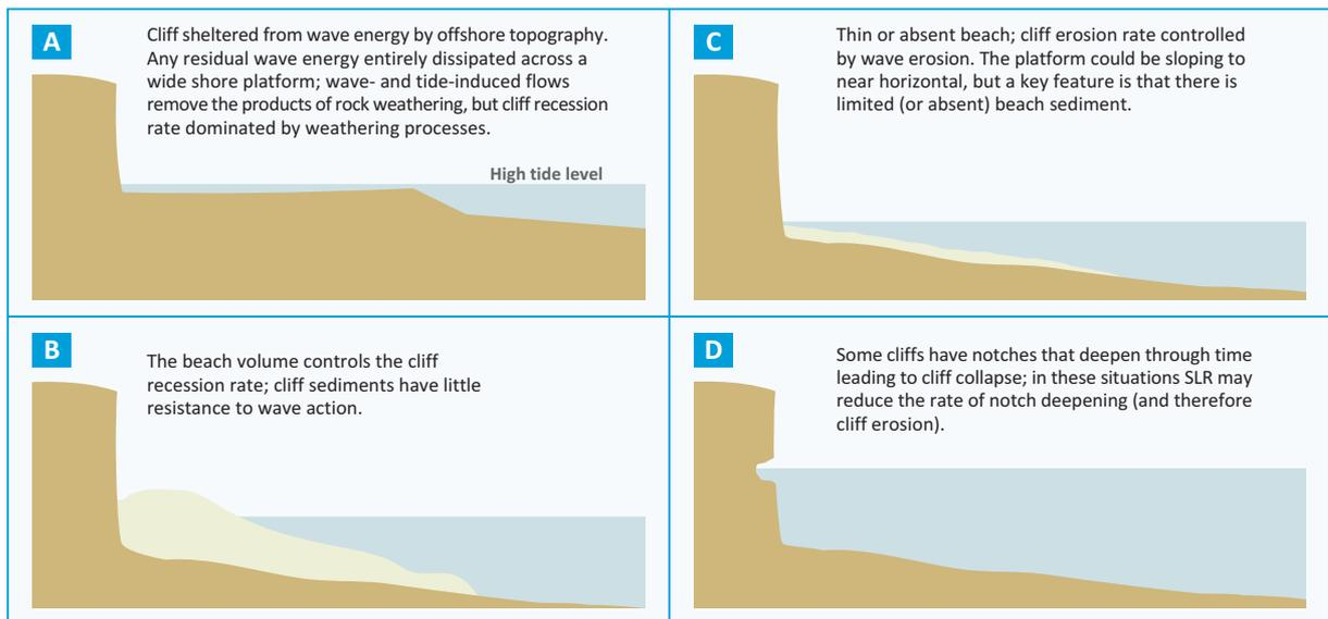
Figure 1: Cliff geometries associated with four possible SLR feedback systems.
