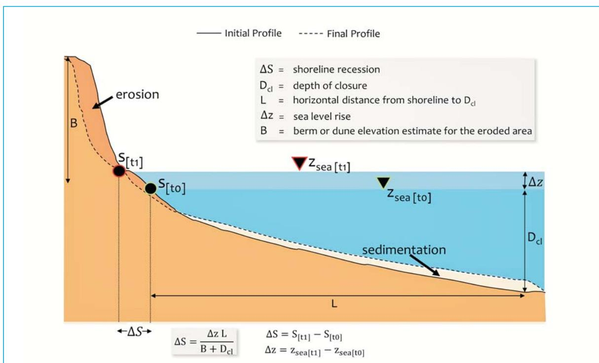
Figure 1: Schematic of the Bruun Rule. Red and green symbols refer to the initial and final conditions, respectively.
