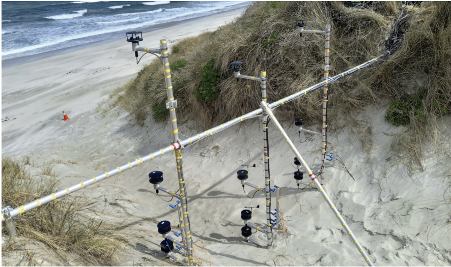
Figure 2: Field-based experiment at Notch C, St Kilda, Dunedin using an array of ultrasonic anemometers (black) and a particle sand counter (LCP) (blue) (Nguyen et al., 2021).
